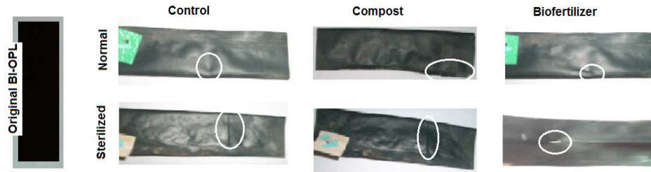
Figure 4: Photographical Comparison between the Different Treatments at the End of Experiment Showing the Cracks of Bi-OPL Tubes (Inside Circles)
